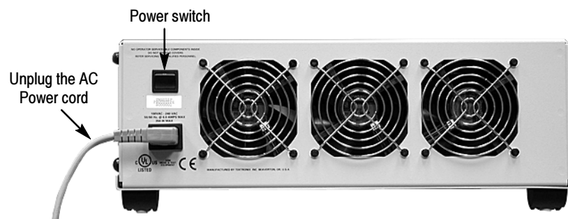
Figure 5-21: Power switch and AC power cord locations
