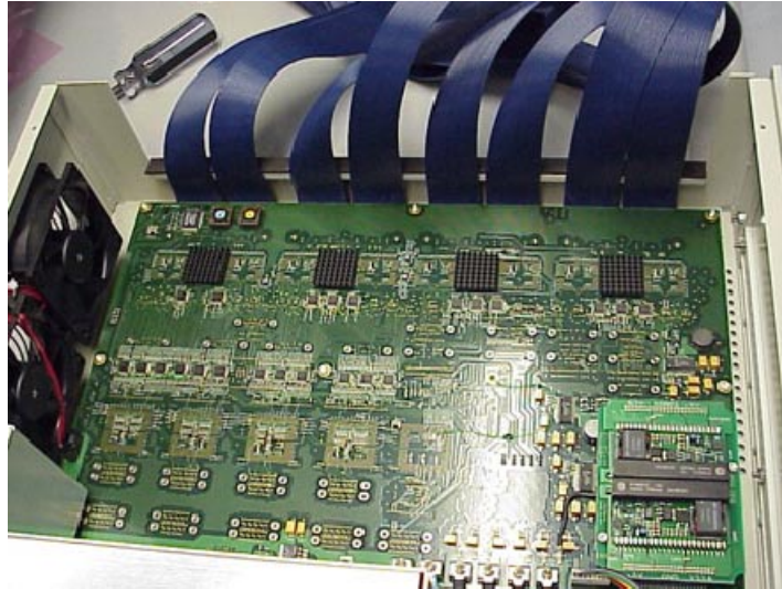
Figure 5-13: Place logic board in the chassis
