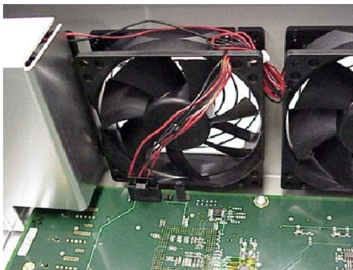
Figure 5-16: Attach fan plug
