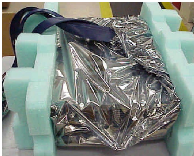
Figure 1-13: Place the end caps on the preprocessor
