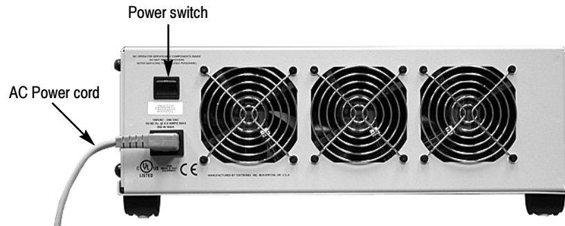
Figure 5-1: Remove AC power cord
