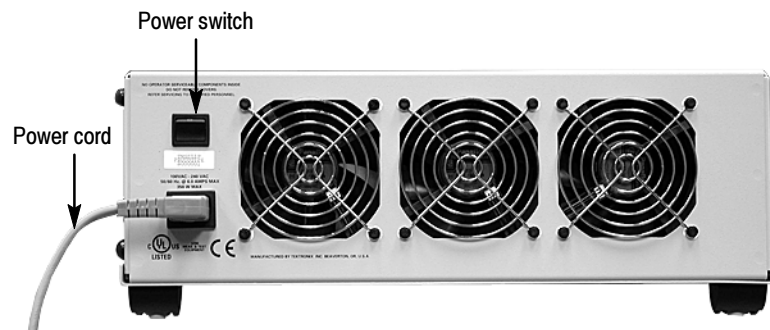
Figure 5-10: Power switch location
