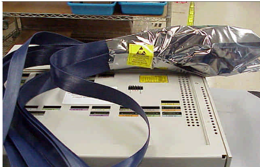
Figure 1-12: Place the probe head in a static shielding bag
